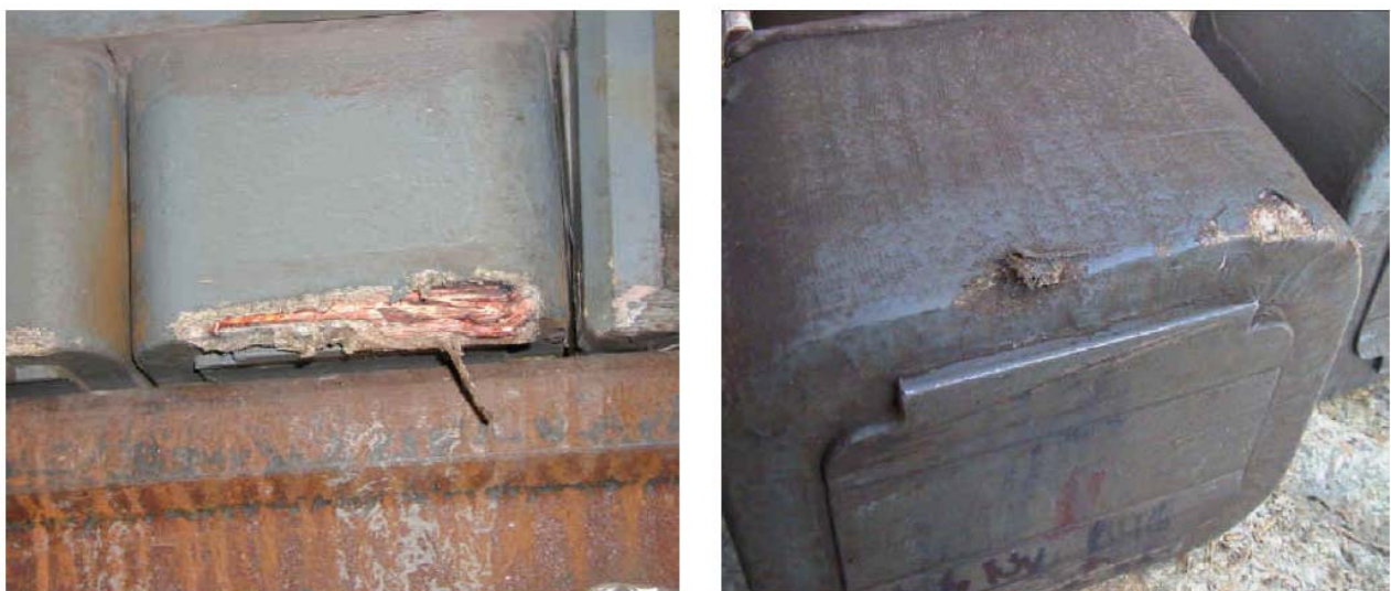
Figure 6: damage to ECB from collision with unknown objects [8]
