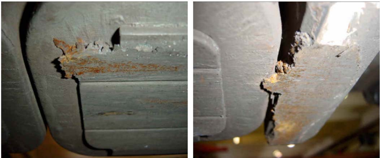
Figure 5: damage to ECB from collision due to insufficiently large air gap [8]
