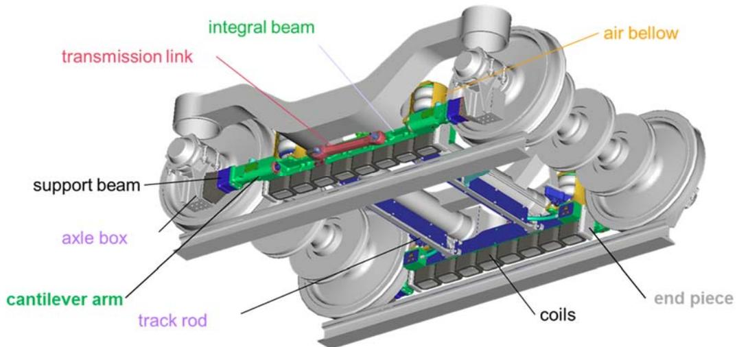
**Figure 1: Main bogie mounted components of ECB**
